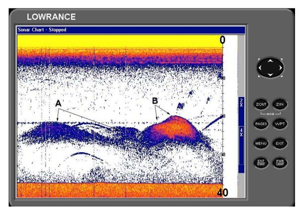
A: & B: Another good contrast of schools of baitfish. A: is faint broken, and shows no color. These bait are closer to the edges of the coverage area than B: which is depicted by a densely packed ball returning a lot of echo signal strength and showing color. Now we begin to see the bait is associating either right at or just below the thermocline. We can only guess if the bait are being driven up into the thermocline or down into it by the game fish, but at the thermocline they are.
