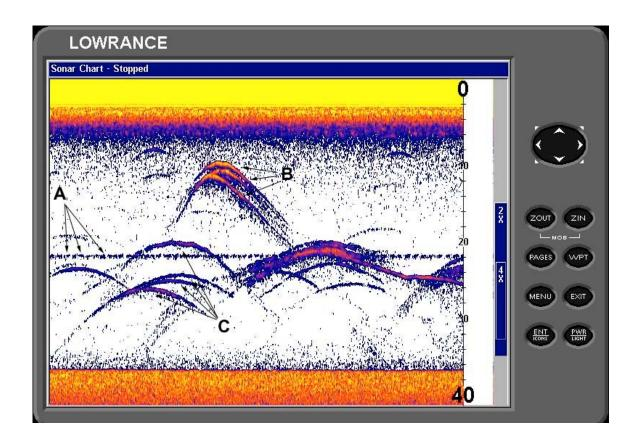
**A**: Depicts the thermocline. In this portion of the chart it is easily seen, in others it is not. You may have begun to notice that most of the activity is very close to this thermocline. This chart also shows active fish (**B**:) closer to the surface which streak away when we reach a distance of approx. 10 feet from them. Other deeper inactive fish (**C**:) are not disturbed by our trolling approach.
