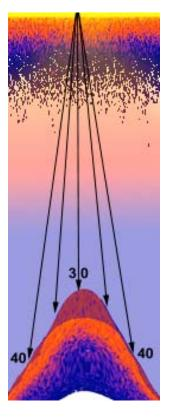
While you may begin to pick up the slightest echo returns from suspended targets which are farther away than the bottom, they do not chart on the screen until they are closer than the bottom as no details are plotted below the bottom contour line. The shape and strength of an echo arch can provide clues to where it is located relative to the center or nearest point of the transducer.
