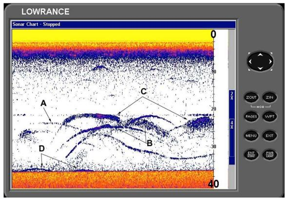
A: Indicates the beginning of a track made by an active and moving fish. The "arch", if we can call it that, shows that although the fish moved a little farther away from the boat it did for a while actually parallel the boat. It may have been inspecting our trolled live bait.
