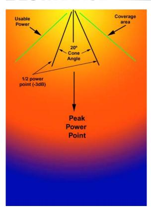
This diagram illustrates the relationship between Cone Angles and coverage areas as well as how this measurement is taken.
