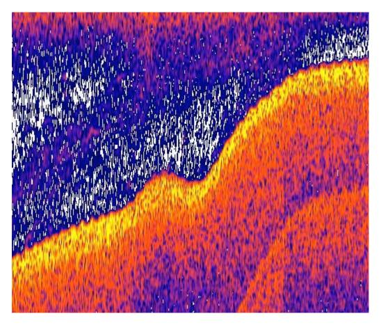
This chart has the appearance of a jagged bottom contour. As if the bottom was chiseled out of splintered stone or growing fissures. In actuality this chart was recorded over a flat, featureless, smooth, hard sand bottom. It was also with a transducer on a very narrow beam aluminum hulled "V" bottomed boat. This boat was prone to a lot of movement and the result is as pictured.
