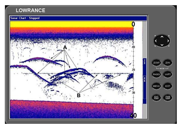
A: This is a prime example of what is referred to as "streaking". This effect occurs when you begin to mark a fish arch, however reach a point where the fish notices the boat shadow, motor, or other stimulus and move rapidly away from the transducer. Remember, although the streaks go down, it doesn't mean the fish moved deep, only that they moved away from the transducer. They may have stayed at the same depth and simply showed their tail fins to the boat.
