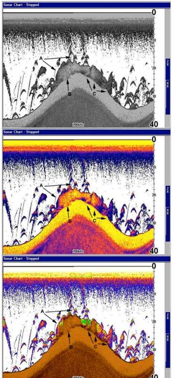
The same chart is pictured here at the same resolution, same sensitivity, and other chart settings. A: denotes suspended targets of bait fish and game fish in and around some type of bottom contact structure. B: indicates structure attached to bottom which is similar in echo return blurring the line between bottom and structure on bottom. C: shows a hard bottom contour indicated by clean hard color separation from structure above.
