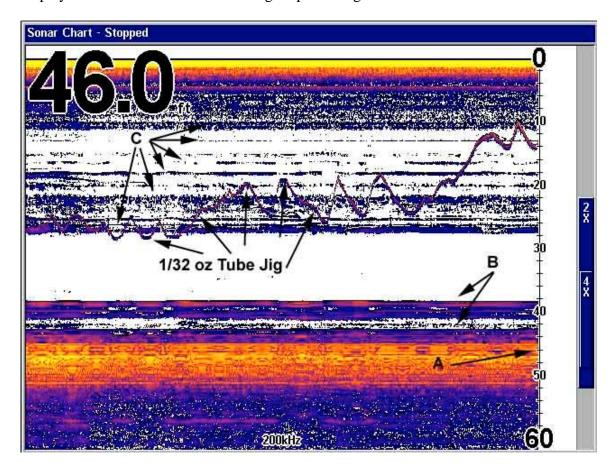
A: Denotes actual bottom under the transducer. B: indicates softer echoes from brush pile directly below the transducer. C: indicates stratified layers of water which are a combination of thermocline and oxyclines. The track going through the chart is a 1/32 oz. Tube jig moving vertically closer and farther away from the transducer.
